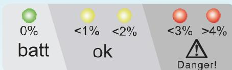
► Quality is tested and indicated on five LEDs in terms of percentage of water in the brake fluid.
