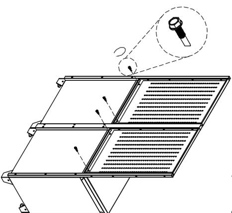
Insert the Hexagon bolt with flange screw(M6X25) through the back of hauger boards, and into the side of SS work plate. Tighten securely.
