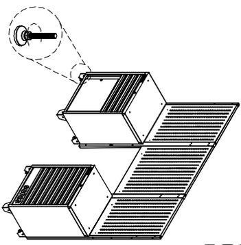
**4. PRE-DRILL HOLES OF SS WORK PLATE**
