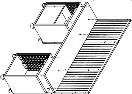
Insert the Hexagon bolt with flange screws (M6X25) through the back of hauger boards, and into the side of SS work plate. Tighten securely.
